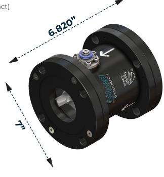
For best results install the Smart Valve downstream of water meter and backflow preventer (if present), but before any other equipment such as a pressure reducer or booster pump. Where possible it is recommended (but not critical) to have 10 diameters of pipe between the water meter and the valve. All flanged installations to use gaskets at each flange.
